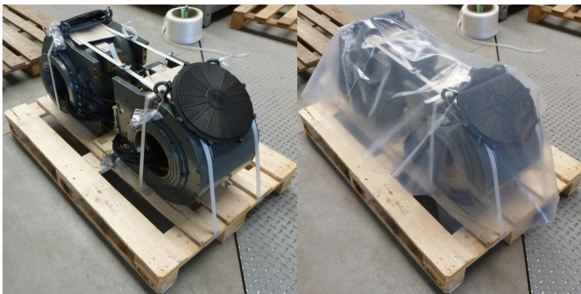
Fig. 55 – Packaging method of 7HLU 3436 P/44-VA motor
