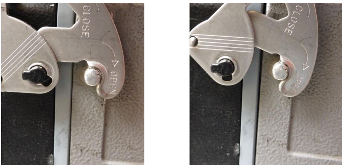
Fig. 54 – Tight seating of the power connector counterpart – GAP IS INADMISSIBLE
