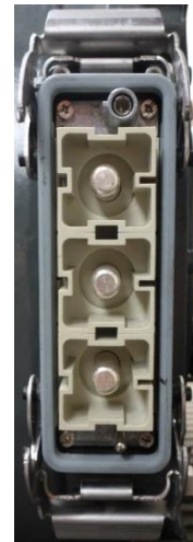
Fig. 52 – Power connector after the removal of protective cap
